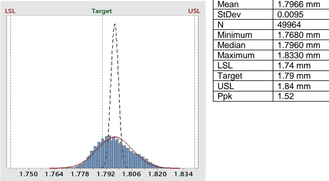
**Figure 1 –** Stratasys ABS-M30 Filament Diameter Analysis
