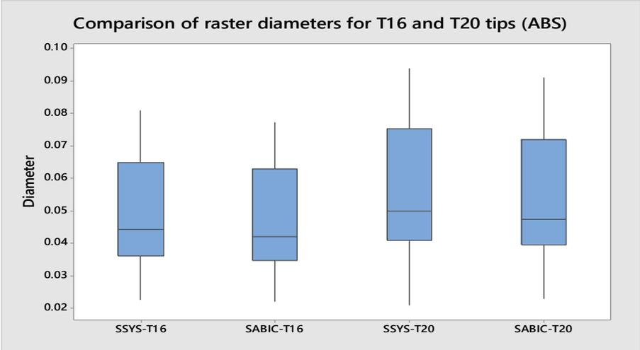
**Figure 3.** Stratasys (SSYS) ABS M30 and SABIC's AMMG94F Filament Extrusion Contour Fill Study
