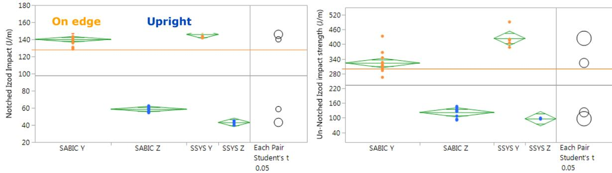
**Figure 9.** Izod (notched and un-notched) impact data for printed specimens
