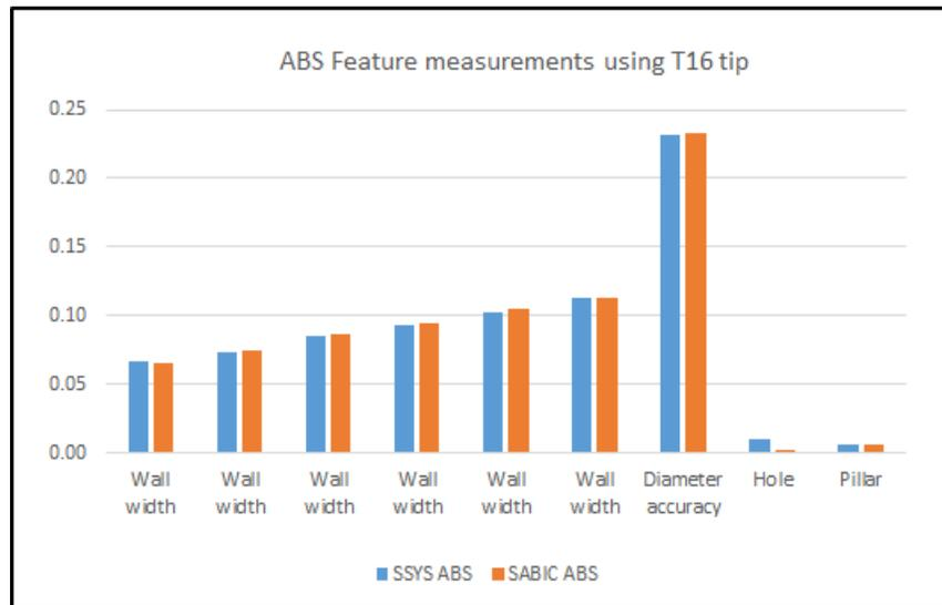
**Figure 5.** Measurements of features printed with T16 tip on Fortus 900mc
