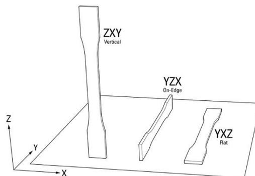
**Figure 6.** Test coupon orientation
