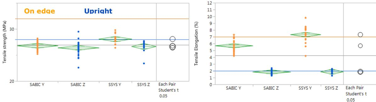
**Figure 8.** Tensile strength and percent elongation for printed specimens
