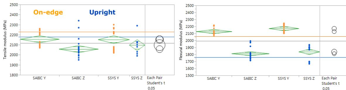
**Figure 7.** Tensile modulus and flexural modulus for printed specimens
